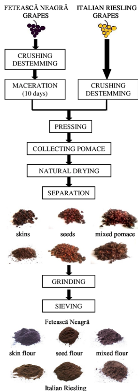
Fig. 1 Technological process of obtaining the grape pomace flours from Feteasca Neagra and Italian Riesling
